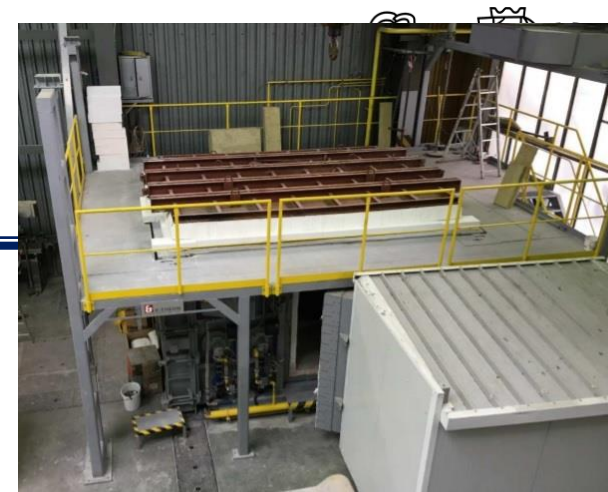
Horizontal furnace in Pavus a.s.
